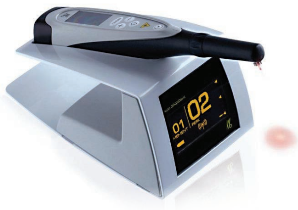
Figure 3: The KaVo DIAGNOdent pen. A hand-held device for caries detection using laser-induced fluorescence.
