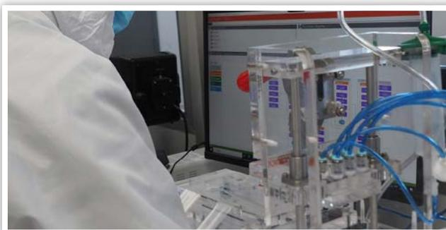
Pressure test to detect leaks in the devices.
