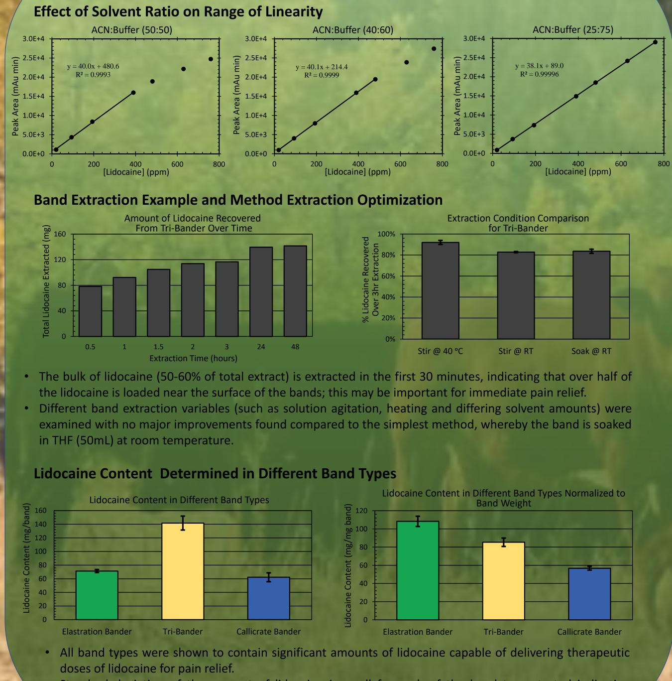
• Standard deviation of the amount of lidocaine is small for each of the band types tested indicating manufacturing process is reliable and repeatable.
