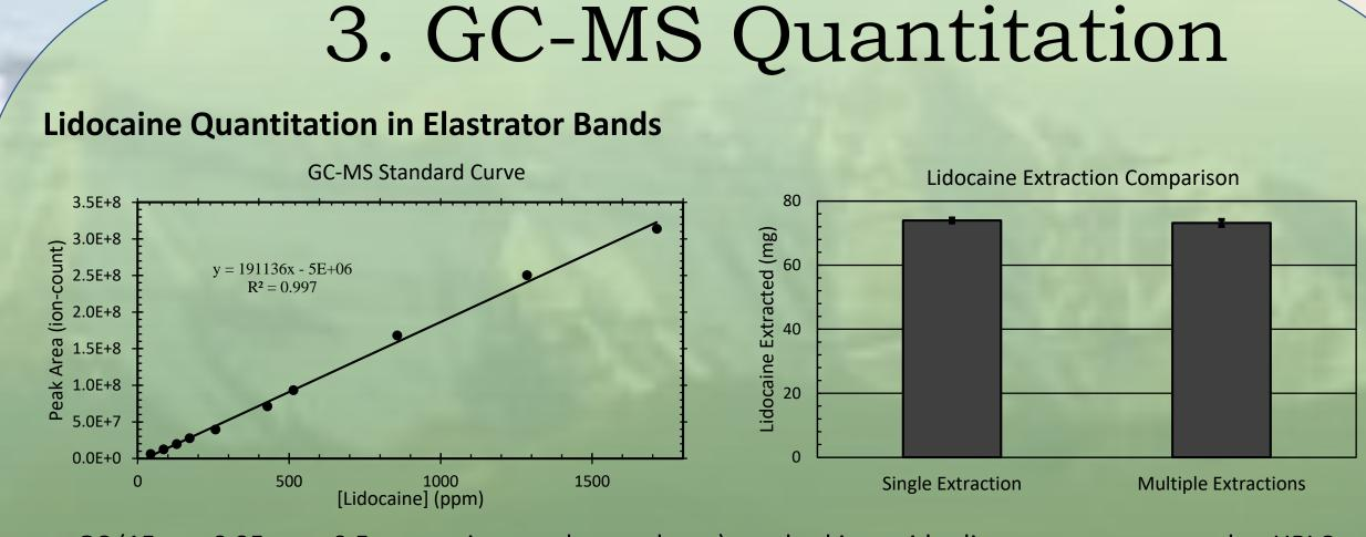
• GC (15 m x 0.25 mm, 0.5 µm stationary phase column) resulted in a wider linear range compared to HPLC. • Extracting lidocaine once compared to multiple extractions (x3), over the same time period, resulted in the same amount of lidocaine recovered (73.93±0.71 mg/band and 73.16±1.04 mg/band respectively).
