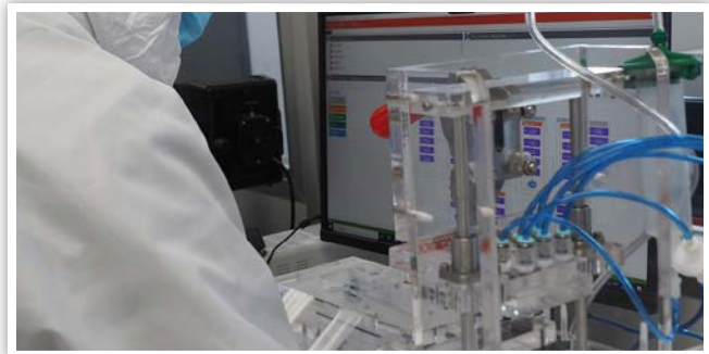
Pressure test to detect leaks in the devices.
